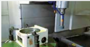
Finishing grinding for casting ID
