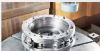
Finishing grinding for brake drum face+ID+OD
