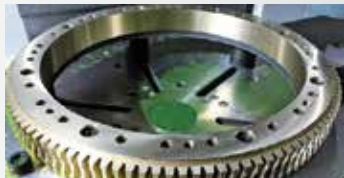
Finishing grinding for gear face
