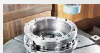
煞車環端面+內外徑研磨
